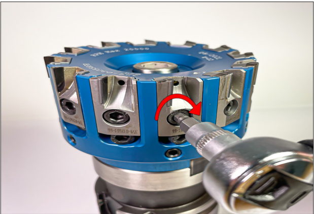
6. Tighten the cartridges to a torque of 12Nm (check that the presetting is correct).
