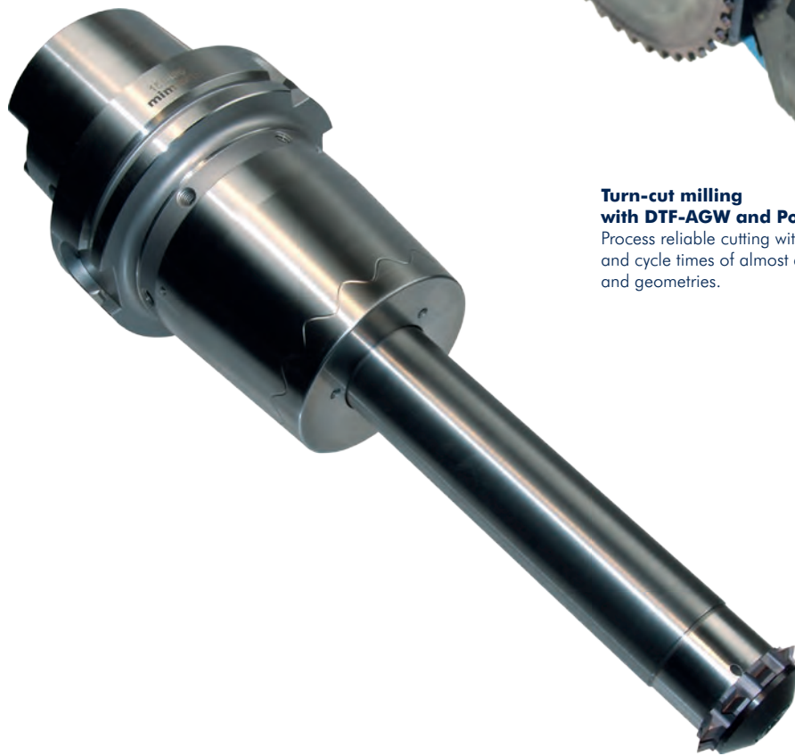
Large thread milling M330x6 with STC1 Material: S355JR
