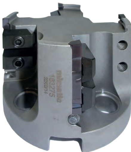
Countersinking and circular milling of a brake body with DE inserts Material: GGG50
